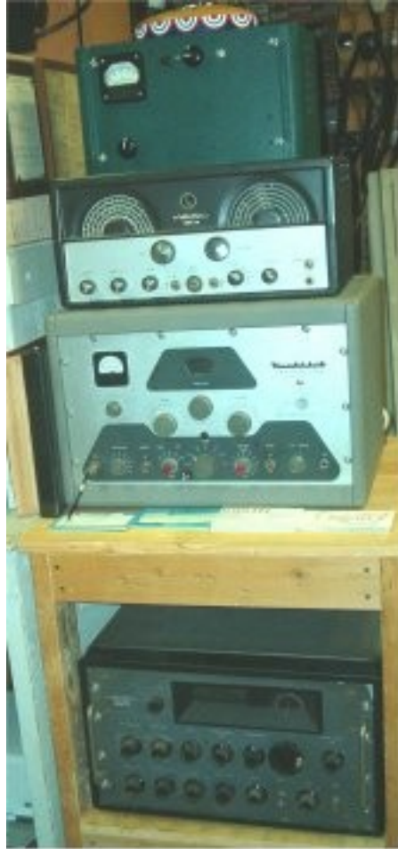
From bottom to top: Hallicrafters HT-20 transmitter; Heath DX-100 transmitter; Hallicrafters S-85 receiver; home brew 222 MHz linear amplifier (100 watts output).
